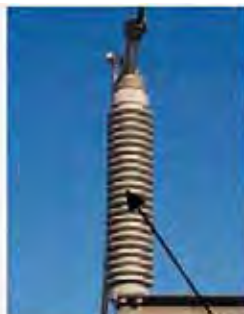
Ceramic Stress Tracking - Corona
